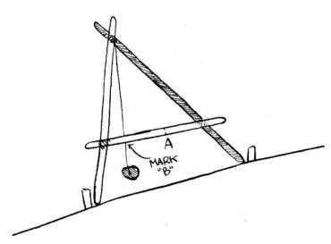
Fig. A2.11. Calibrating the A-frame, step two
