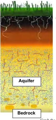
Underground layers of clay, sand, gravel, and rock that can store water.
