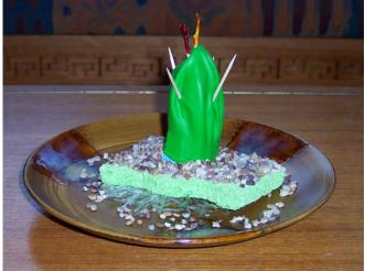
the sponge is saturated and there is a small pool of water on the plate. (Note: a spray bottle can be used instead of a measuring cup to better simulate rain, but the process of saturating the sponge will take much longer.)
