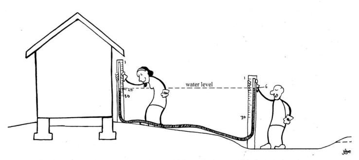
Fig. A2.7. Using a bunyip to measure how much lower the bottom of the basin is than the area near the house, confirming that the slope now drains away from the house
