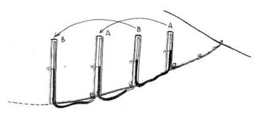
Fig. A2.5. Leapfrogging the bunyip to mark a level contour line on the land. Here the contour line is marked both by scuffing a line in the dirt and with stakes.
