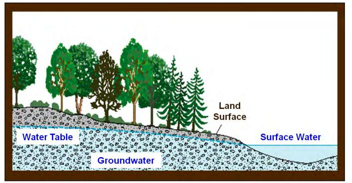
Groundwater fills the spaces between soil particles and fractured rock underground.
