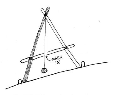
Fig. A2.10. Calibrating the A-frame, step one
