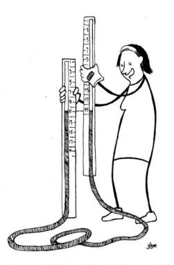
Fig. A2.2. Testing the bunyip level; the water is level.
