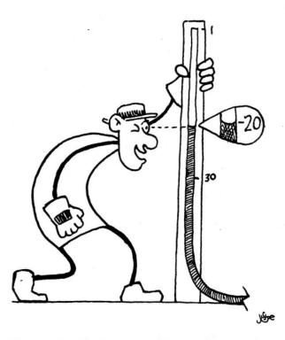
Fig. A2.4B. The bunyip stake must be vertical for a correct reading
